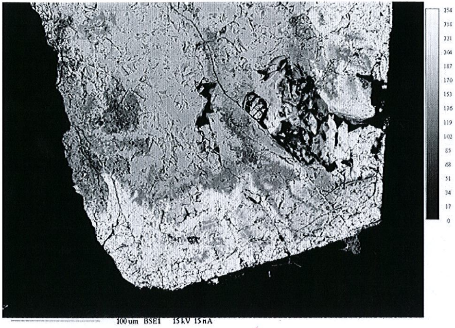
Fig. 3. BSE image of pyrochlore from the Gjerdingen ekerite. Detail of the lower right part of Fig. 1.
