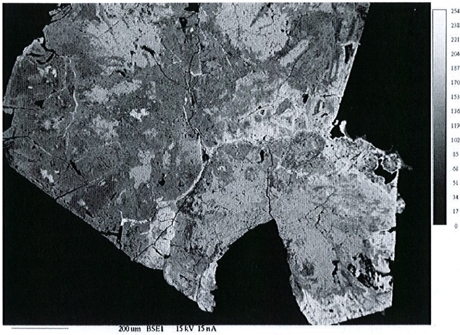
Fig. 1. Back-scattered electron (BSE) image of two intergrown pyrochlore crystals from the Gjerdingen ekerite. Details of the lower parts are shown in Figs. 2 and 3.
