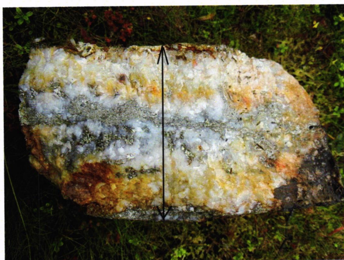
Fig. 6. A complete cross-section of quartz vein #1, approximately 20 cm wide (shown by arrow).
